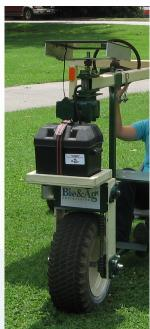
Garden Scooter 1.0 is battery powered, solar assisted and made entirely of recycled or salvaged parts. The back wheel assembly is adjustable to accommodate varying row widths.
