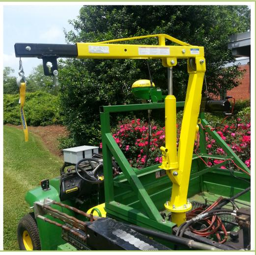
The Electric Jib Crane was designed for producers with lifting limitations to assemble their own adaptive solution by utilizing common, commercially-available components to assist farmers with everyday tasks such as loading or transferring loads. This idea was inspired by a NC AgrAbility farmer/veteran with a UE amputation. A publication on this design is available for free to the public at http://www.bae.ncsu.edu/extension/ext-publications/#agricultural
